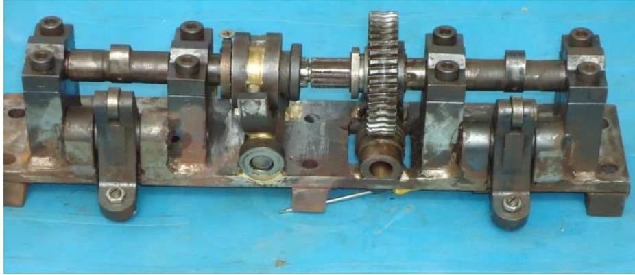
**Figure 7.** The mechanism for controlling cylinder deactivation
