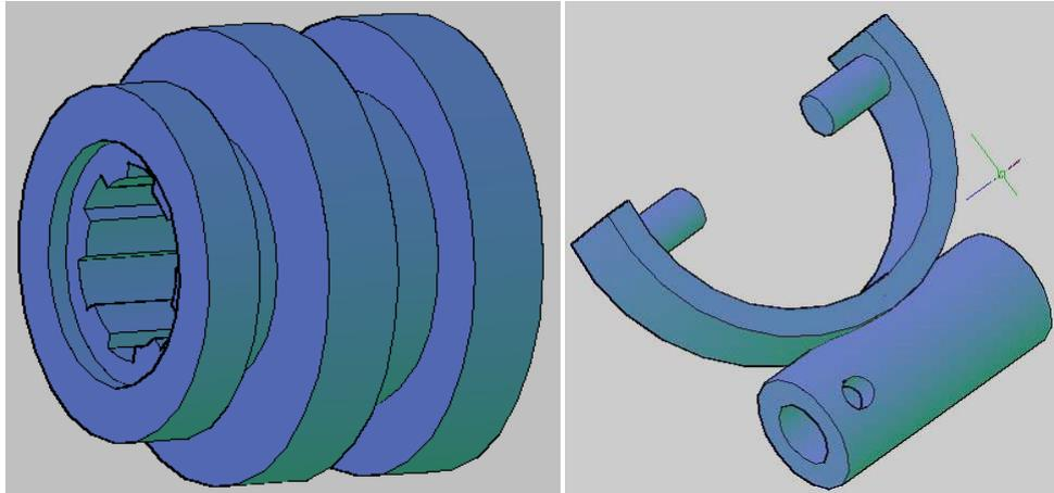
**Figure 5.** The splined joint and controlled fork
