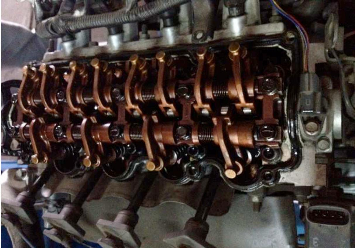
**Figure 2.** The conventional valve train system in Hyundai engine G4EK
