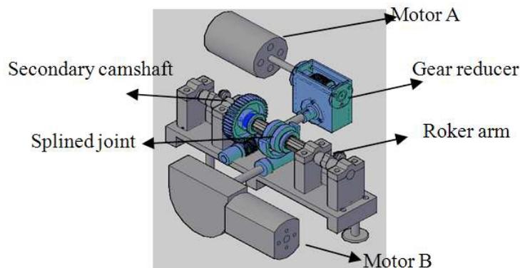
**Figure 6.** The cylinder deactivation control mechanism diagram
