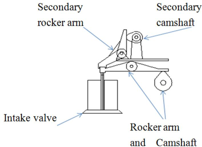
**Figure 3.** Intake valve control mechanism for cylinder deactivation
