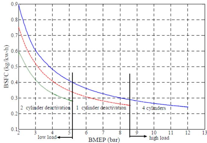
**Figure 9.** Effects of cylinder deactivation at entire load ranges
