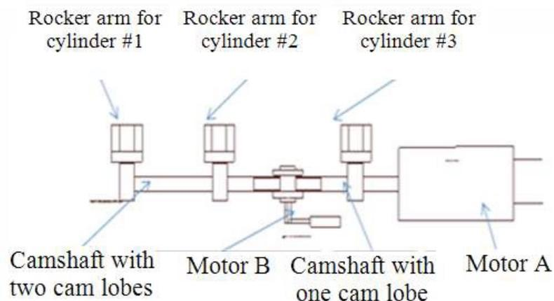
**Figure 4.** The outline of cylinder deactivation mechanism
