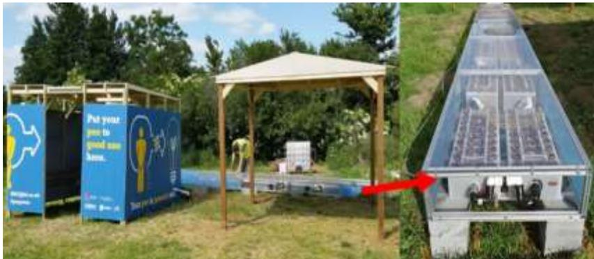
**Figure 2: MFC Module assemble outside**
