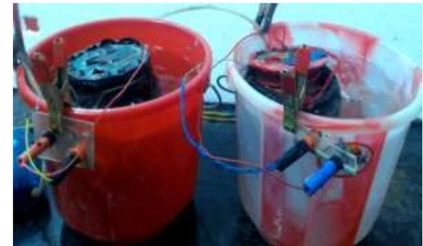
**Figure 3: Dual Chamber MFC (batch mode)**
