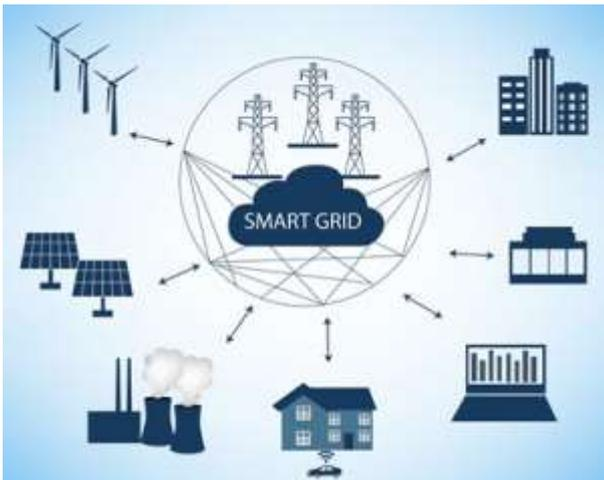
Most grids are based on one-way interaction from the stages of generation to consumption. Smart grids, on the other hand, integrate the action of all users in the power network using computer-based remote control and automation. This two-way interaction is what makes the grid “smart”. Like the internet, the Smart Grid consists of
