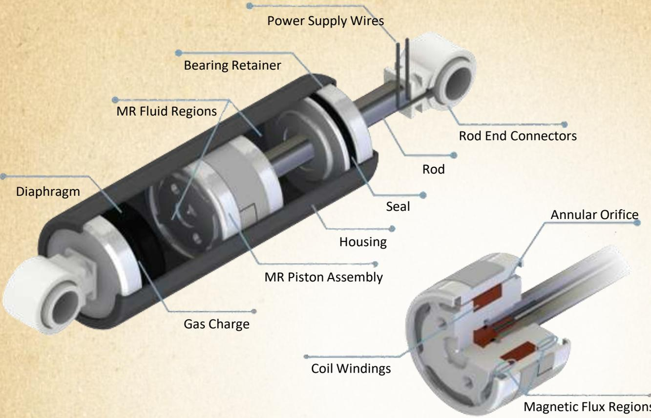
Application of MR fluid in vehicle dampers to absorb impact forces in suspension
