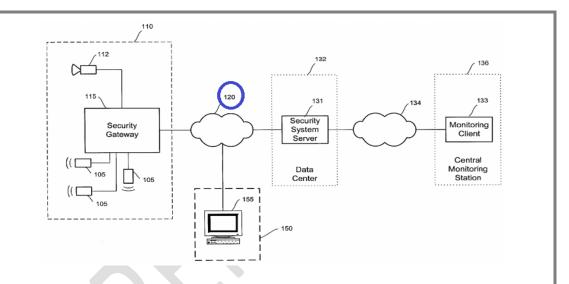
[Para 33] In general, network 120 may be a public network or private network, a single network or a combination of several networks. In most embodiments, network 120 may be, but is not required to be, an IP-based network. In some embodiments it may be desirable for all or a portion of network 120 to include publicly available networks, such as the Internet, to avoid the need for installing, purchasing, or leasing additional infrastructure.
