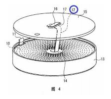
End portion of second electrode is connected to bottom metallic housing part
