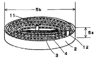
**Searcher's Comment:** Unlike the proposed invention, both ends of the jelly roll is connected to the upper housing part.
