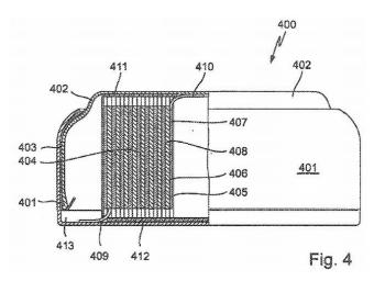
The electrode-separator assembly is packed in the metallic hosing parts (button cell) and is sealed using adhesive sealant
