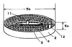
End portion of second electrode is connected to bottom metallic housing part
