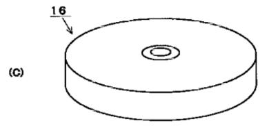
An electrode-separator assembly comprising an insulator placed as separator in between flat positive and negative electrodes
