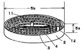
The electrode-separator assembly is aligned perpendicular to the surface of button cell
