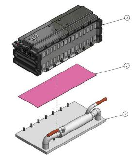
Prototype Isothermal base cooling solution
