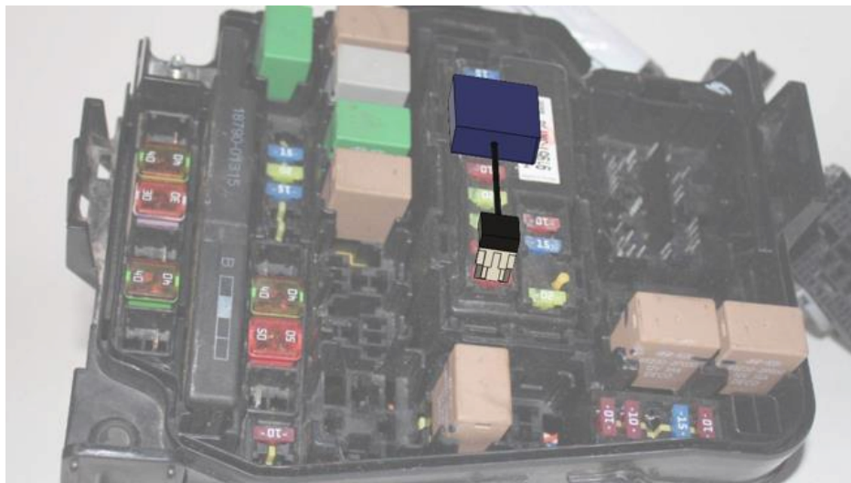
EngineLock SM installed in ECU slot in under hood fuse box
